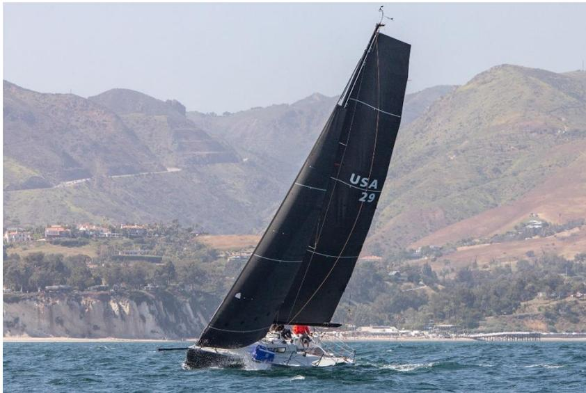
BeetleCat, sail USA 29 with an off-wind performance handicap for this race of a 60 rating, is a matte-black ultralight 29-foot Bravura B-29 sloop with a black flat top main and jib. Great in light air, but not great at drifting.
